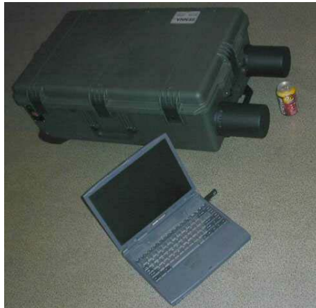
Figure 6. SENNA – portable sensor for explosives' detection based on Nanosecond Neutron Analysis.
